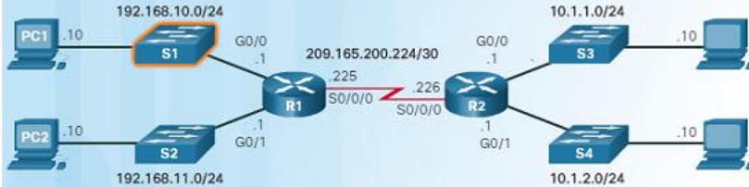
Configure the Switch Management Interface
