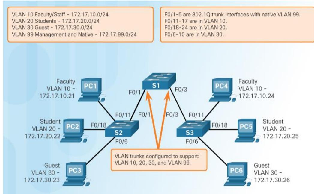
The links between switches S1 and S2, and S1 and S3 are configured to transmit traffic coming from VLANs 10, 20, 30, and 99 across the network.
