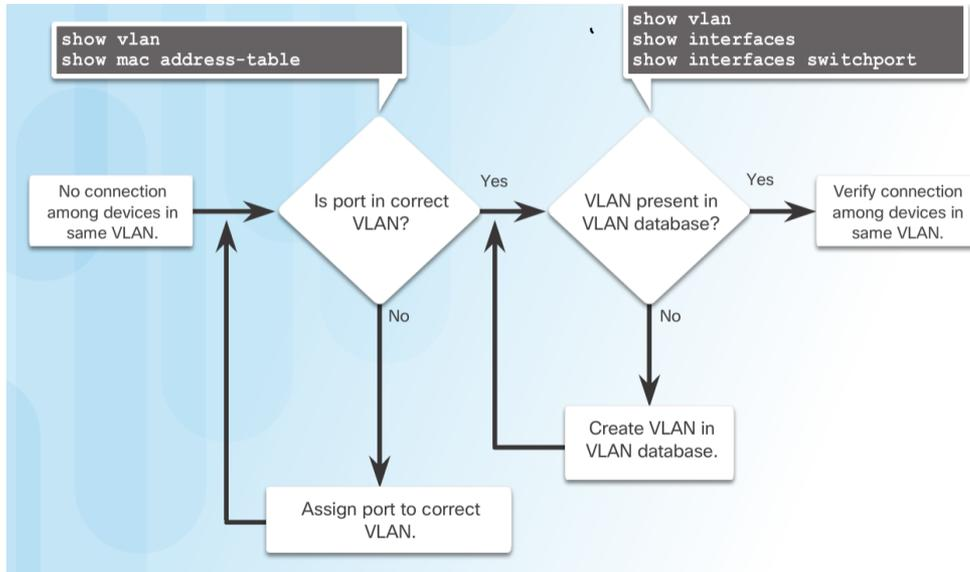
If the VLAN to which the port belongs is deleted, the port becomes inactive and is unable to communicate with the rest of the network.
