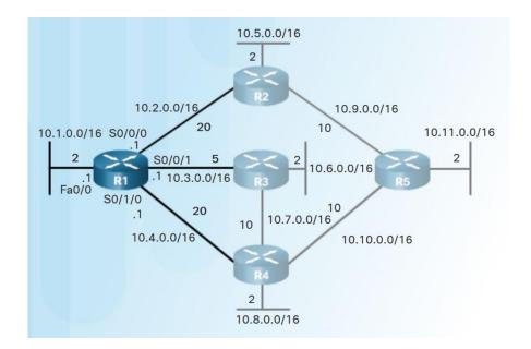
The first step in the link-state routing process is that each router learns its own directly connected networks.
