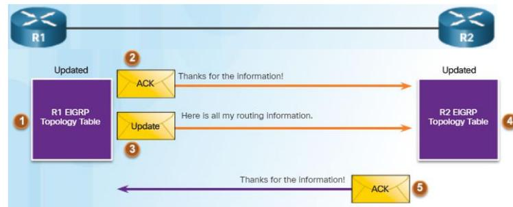
2. EIGRP update packets use reliable delivery; therefore, R1 replies with an EIGRP acknowledgment packet informing R2 that it has received the update.
