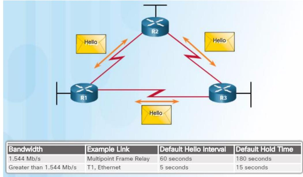
EIGRP uses multicast and unicast rather than broadcast.
